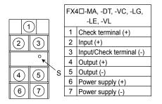
S: FX4□-MA; Moving average time setting volume FX4□-DT; Dead time setting volume FX4□-VC; Velocity computation time setting volume FX4□-LG, -LE; Time constant setting volume
